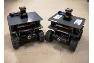
Fig. 3. (left) The proposed map fusion algorithm. Two input maps, map_1 and map_2 , are fused by finding their relative transformation matrix. No prior information is available regarding the relative position of two respective robots. (right) Experimental robots, CoroBot, each equipped with a laser ranger and wheel encoders.
