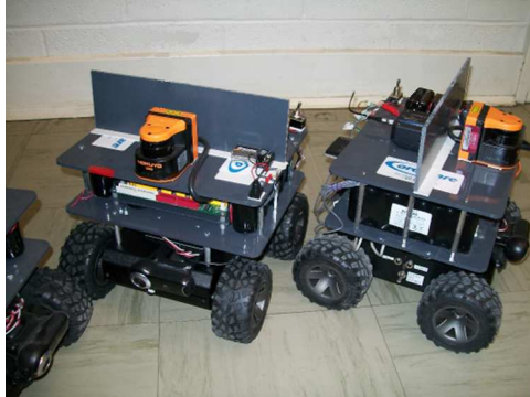
Figure 8: Robots equipped with the laser rangefinder, MEMS IMU and wheel encoders (not visible)
