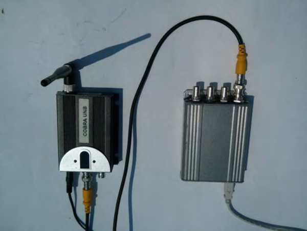
Fig. 4. A wireless receiver (left), and a frame-grabber (right) are used to receive the imagery data.
