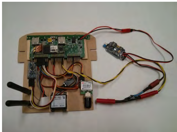
Fig. 2. Onboard sensors and the processing unit. As shown in the figure, the IMU, GPS, and pressure data are captured by the processing unit and sent to the GCS using the WiFi channel. (Camera is not shown in this figure).
