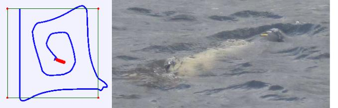
Fig. 11. The path planned by the proposed planner for a for a square workspace with constant and *a priori* known parameters (left). The IVER2 AUV made by OceanServer Technology used for trials (right).
