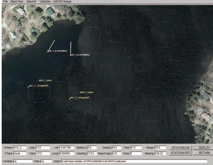
Fig. 7. A screenshot of the *pMarineViewer* application with two AUVs shown.
